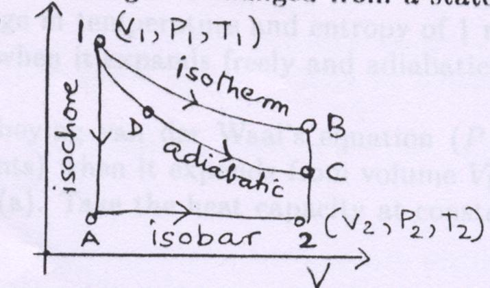
$(P_2, V_2, T_2)$  by the following three quasistatic processes as seen in the figure: (i)1A2 (ii) 1B2 and (iii) 1DC2. What is the increase in internal energy for  $1 \to 2$ ? Also obtain the work that must be done on the system and the heat that must be added in each process. Assume that the specific heat at constant volume  $C_V$  is constant and  $\frac{C_P}{C_V} = \gamma$ .
